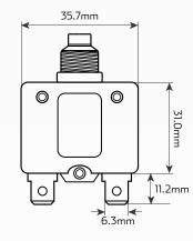
\* Minimum 10mm diameter mounting hole.
