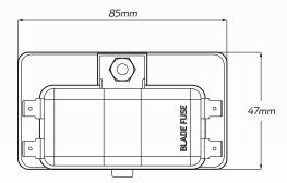
Unit tolerance: +/- 1mm Terminals size: 6.3mm +/- 0.5
