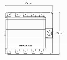
Unit tolerance: +/- 1mm Terminals size: 6.3mm +/- 0.5
